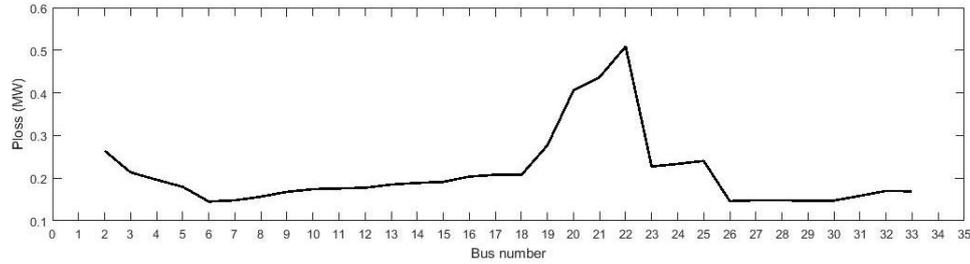
Figure 3.  $P_{loss}$  after individual DG placement at every bus
