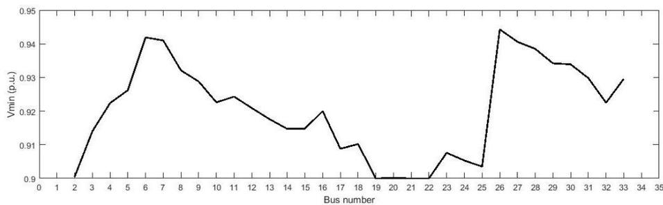
Figure 2.  $V_{min}$  after individual DG placement at every bus
