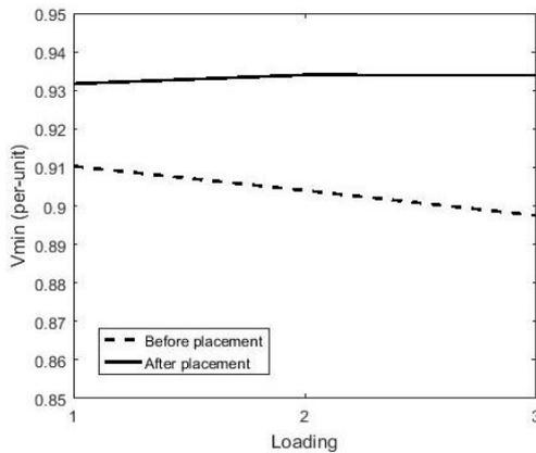
Figure 4. Voltage improvement under various loadings
