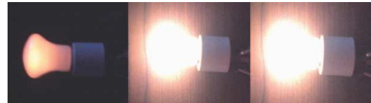
Figure 14. Bulb responses for control value DN = 5, 15, 25
