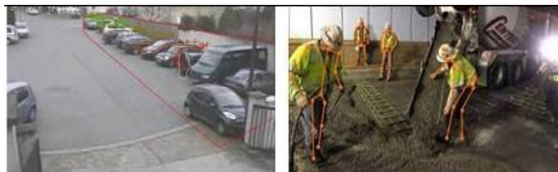
Figure 2. Action recognition from image. (a) Zigzag movement in a car park as a sign for possible car theft and (b) detection of employee's behaviors on site
