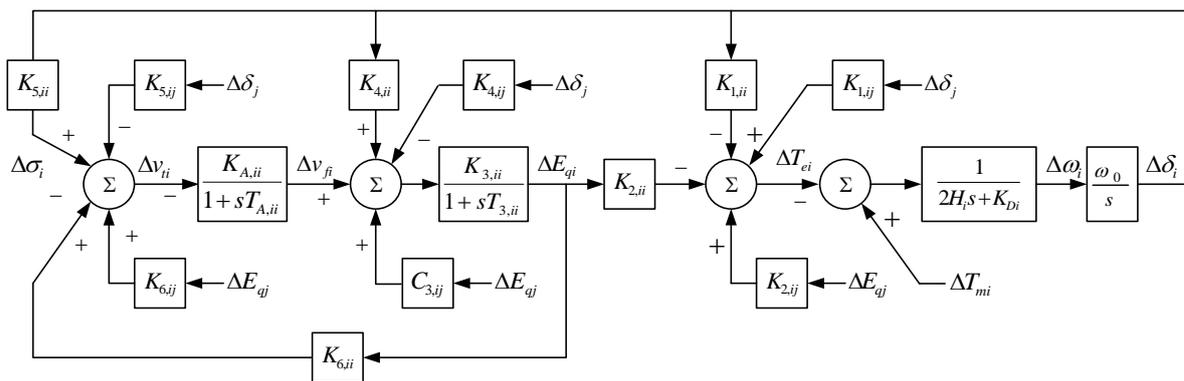
Figure 1. Phillips-heffron model for multi-machine system
