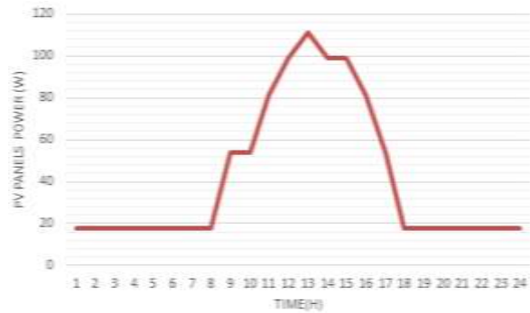
Figure 5. PV panels power fluctuation
