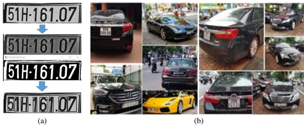
Figure 6. Result of detecting license plate in the second phase, (a) process of detecting characters and digits, (b) different cases of test sample
