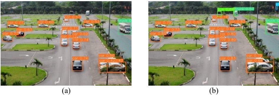
Figure 6. Small object detection results in remote sensing images in Thai Nguyen, Vietnam: (a) detection results based on the YOLOv11 model and (b) detection results using YOLOv11 combined with the SAHI technique using the image slicing method
