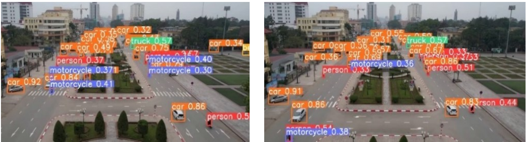
Figure 7. Sample object detection results of YOLOv11 with SAHI on UAV traffic data in Thai Nguyen, Vietnam
