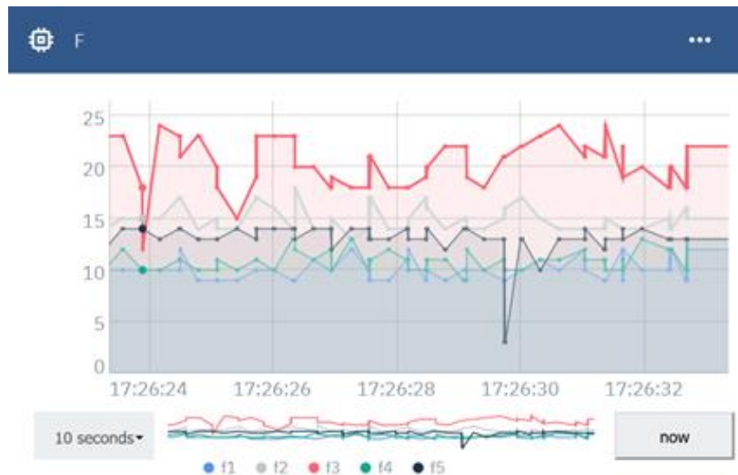
Figure 5. Visualization of flex sensors from glove on IBM Watson IoT platform
