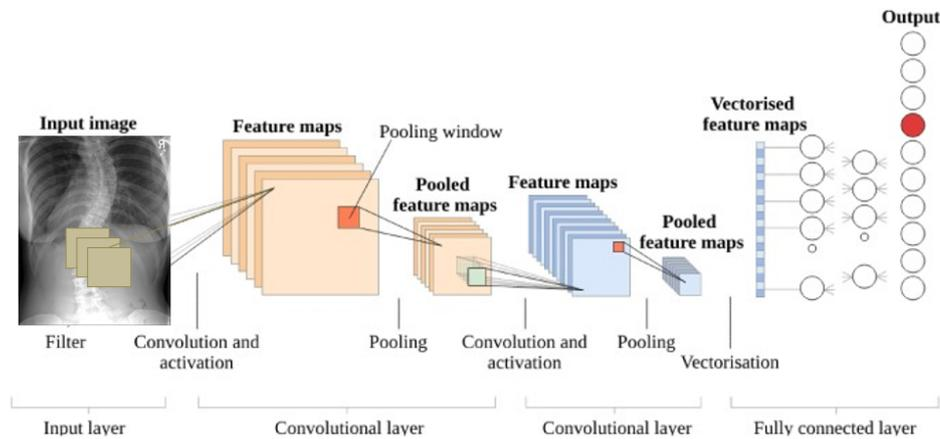
Figure 7. CNN's architecture
