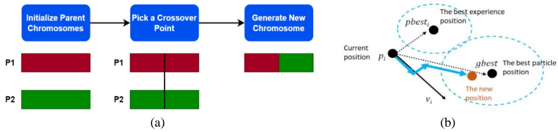
Figure 6. Basic operational principles of two algorithms: (a) major steps for GA and (b) moving particles in PSO
