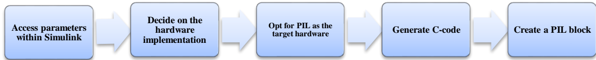
Figure 12. The process for setting up a parameterized PIL test using the LaunchPad F28069M
