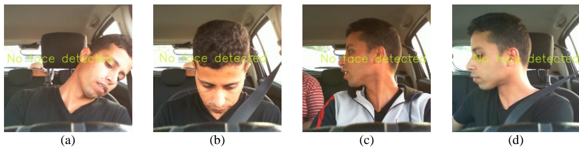
Figure 7. Other situation of driving behavior detection: (a) in-motion no face detected, triggering emergency ADAS warning, (b) moving driver unresponsive, activating emergency ADAS alert, (c) stationary no face detected, no alarm, and (d) stopped driver absent, no alarm
