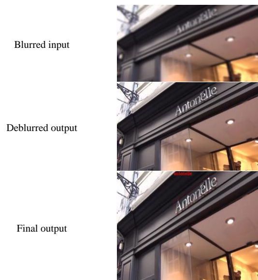
Figure 5. Applied deblurring, text detection and recognition approach at blurred frames
