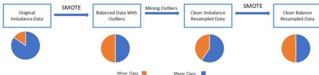
Figure 2. An overview of the RO-SMOTE mode, illustrating the steps and both the minor and major classes involved in each step
