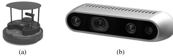
Figure 2. Experimental setup (a) mobile robot platform and (b) intel realSense D435i RGB-D camera
