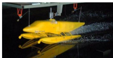
Figure 1. Towing tank test of an amphibious aircraft
