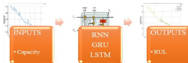
Figure 4. The proposed framework to predict RUL of battery lithium-ion
