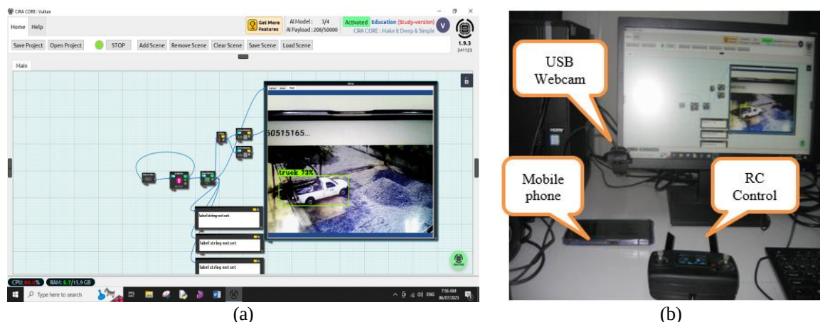
Figure 11. Real-time drone flight control and target object detection system of (a) real-time object detection in the CiRA CORE program and (b) experimental setup and radio control operation in target area 1
