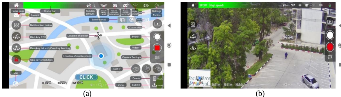
Figure 9. Display on mobile phone of M RC Pro application for drone of (a) application interface with control options and map view and (b) live video feed from the drone's camera shown on the mobile phone
