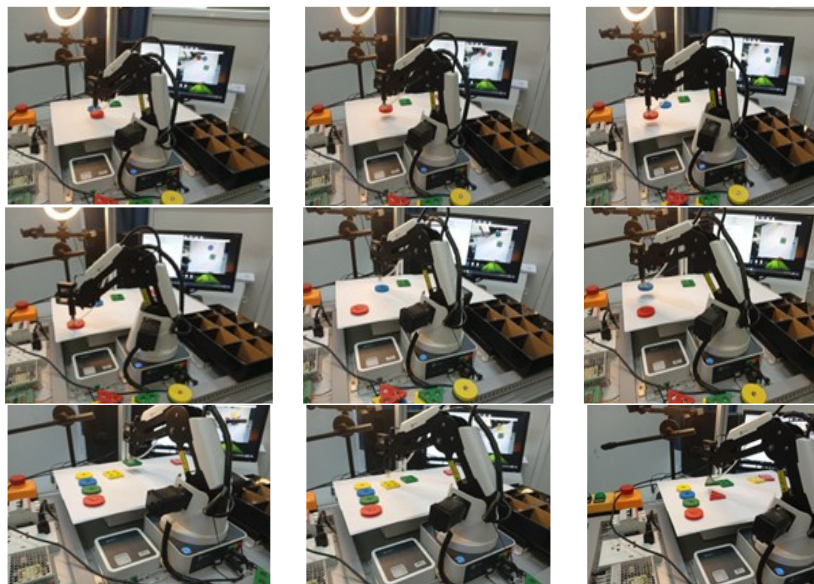
Figure 10. Actual movement of the Dobot Magician during object sorting
