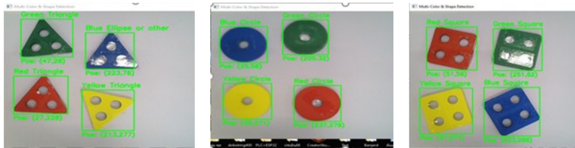
Figure 9. Object detection by shape and color using HSV and OpenCV
