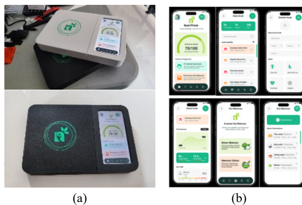
Figure 3. System prototype: (a) hardware unit and (b) Android application interface
