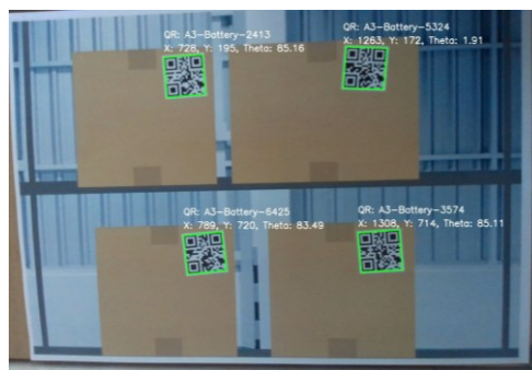
Figure 14. QR-code recognition results obtained by the robot during the automated goods-inspection task, the decoded information corresponds to product identity and location
