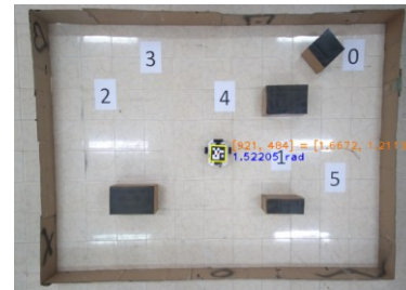
Figure 6. Localization principle using ArUco marker and orientation estimation
