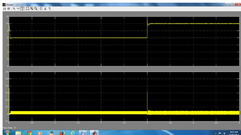
Figure 8. Output of DC-DC (buck) Converter using Proposed NNC
