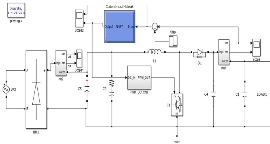
Figure 4. Neural Network Controller for DC-DC (Buck) Power Converter Circuit
